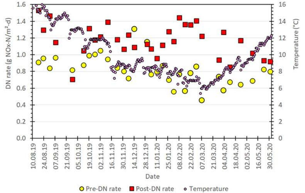
Figure 7 Temperature influence on observed nitrification and denitrification rates at Gardermoen WWTP in 2019 and 2020
