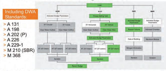
design for several processes of waste water and sludge treatment including equipment
