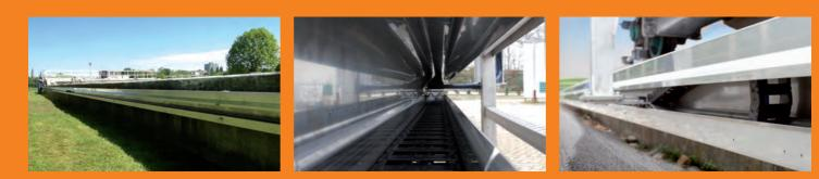
Basic flizz<sup>°</sup> – the energy chain<sup>°</sup> for sewage treatment plants. Watertight housing +++ secure guidance +++ easy assembly +++ simple to retrofit even after installation +++ compact design +++ 200 meter travels and longer possible with igus<sup>°</sup> rol e-chain<sup>°</sup> +++ delivered from stock +++
