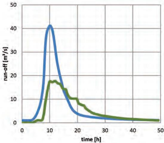
Fig. 2: Comparison of a flood wave of the Emscher tributary, Boye, in the technically developed condition (blue) and the environmentally improved condition (green).
