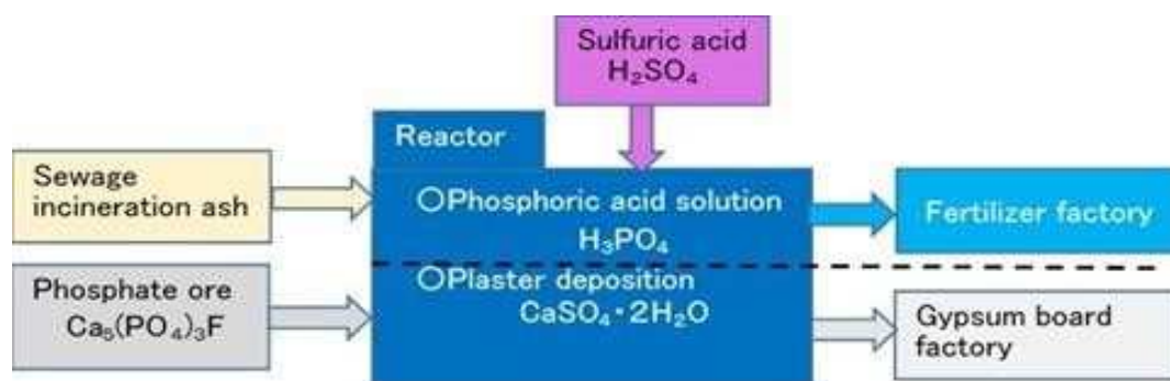
Fig-7 9 Manufacturing process of phosphoric acid and gypsum board
