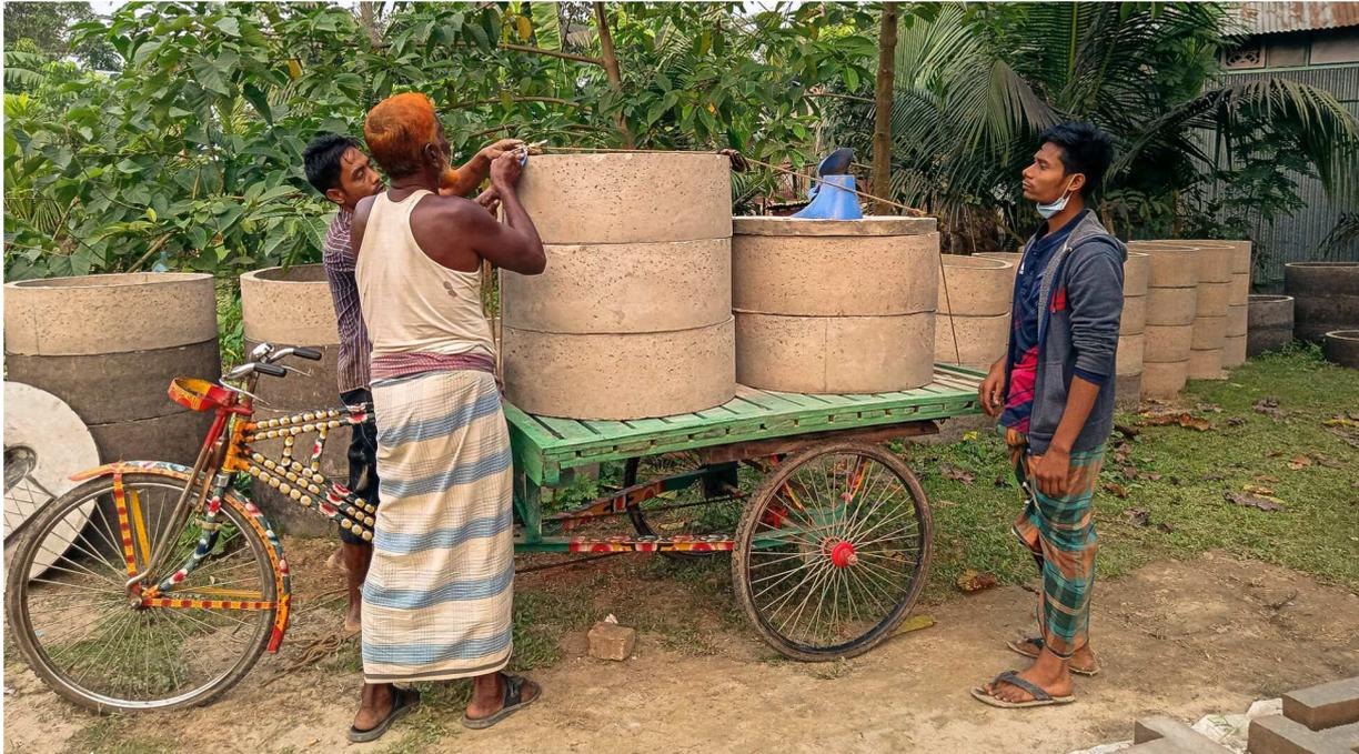
Mubeen, right, learned how to produce “improved latrines” which include cement rings, slabs, and lids, which he is now making at his small factory.
