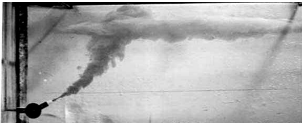
Fig. 4: Laboratory investigation of near-field mixing of submerged discharge into a stratified water body. The initial buoyant jet motion is followed by trapping and internal spreading at the terminal level.
