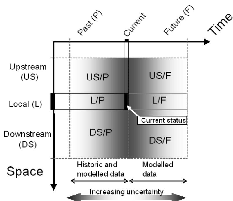
**Figure 4.** Schematic illustration of dynamic water system characterisation. The dynamic characterisation is updated by, and updates, the EIS for different possible action and development scenarios as recent monitoring and interpretation of relevant cause-effect relations changes (EIS, further detailed in Figure 5).
