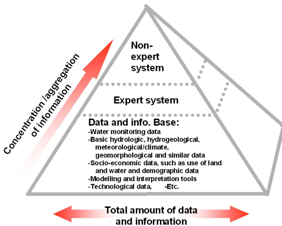
**Figure 5.** Schematic illustration of the generally accessible Environmental Information system (EIS) including a data and information base that contains core data, an expert system for users with necessary knowledge, and a highly aggregated and easily understandable non-expert system.
