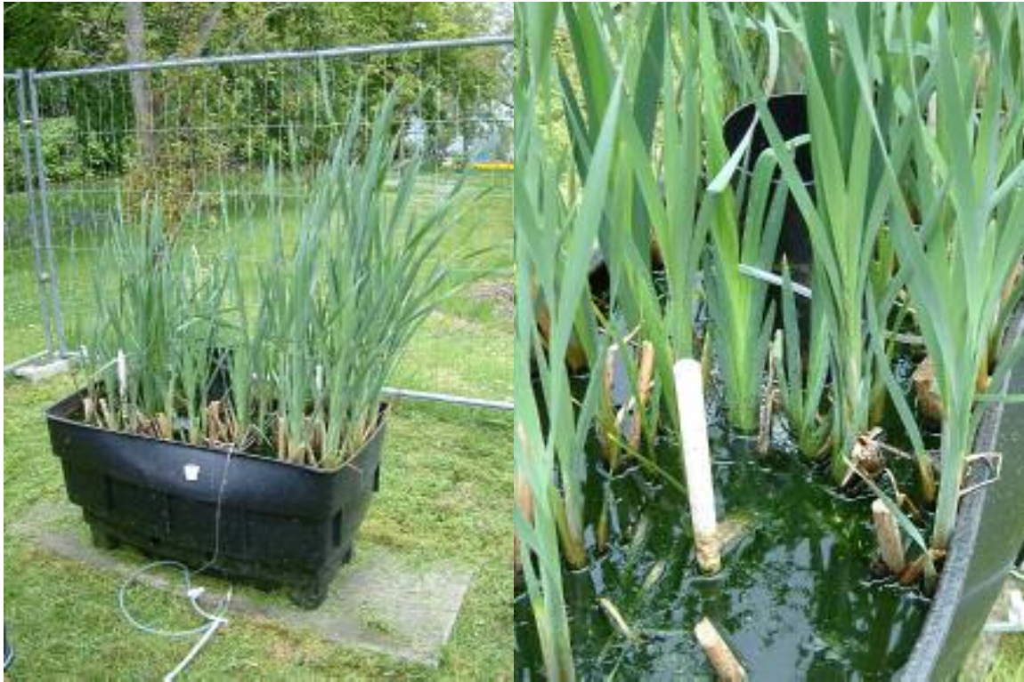
Figure 2: Constructed wetland planted with Reedmace ( Typha latifolia ) on 23 May 2003: a) System overview showing also the aeration pipes fed by an air pump (left picture); and b) System details including the locations of the large outlet pipe and one of the four small aeration pipes (right picture).
