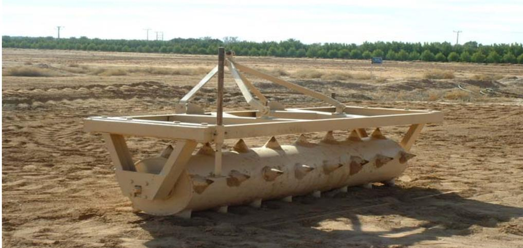
Fig. 1: A designed machine for making pits in the soil surface.
