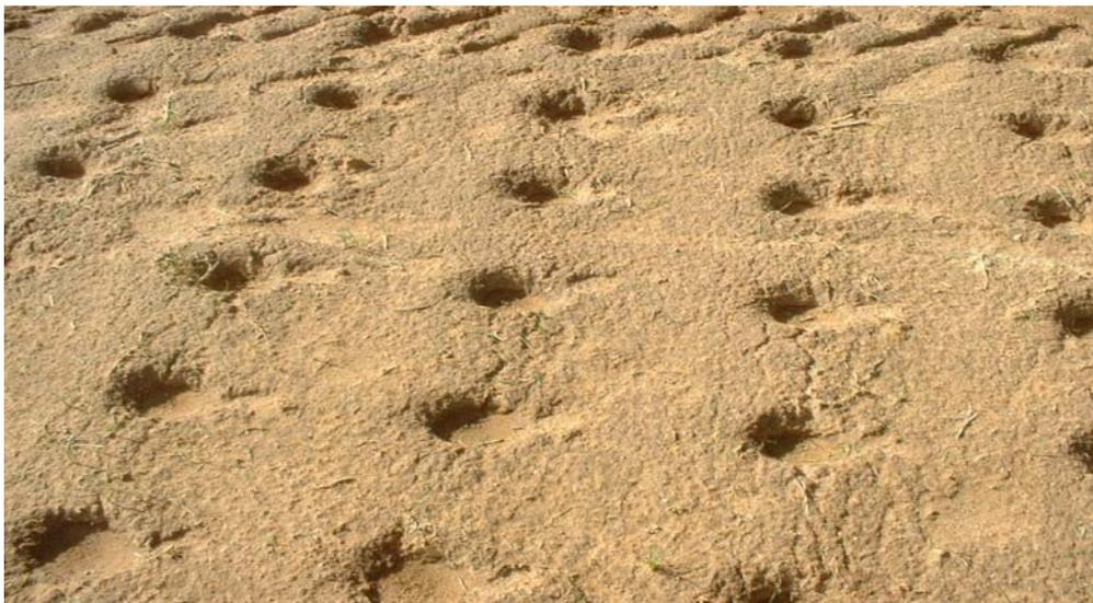
Fig. 2: Pits achieved using the designed machine.
