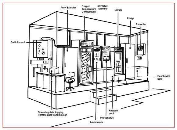
Figure 6: Water Quality Monitoring Station (On-Site Principle).
