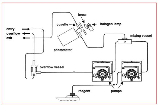
Figure 12: Photometric Measuring Instruments – Principle.
